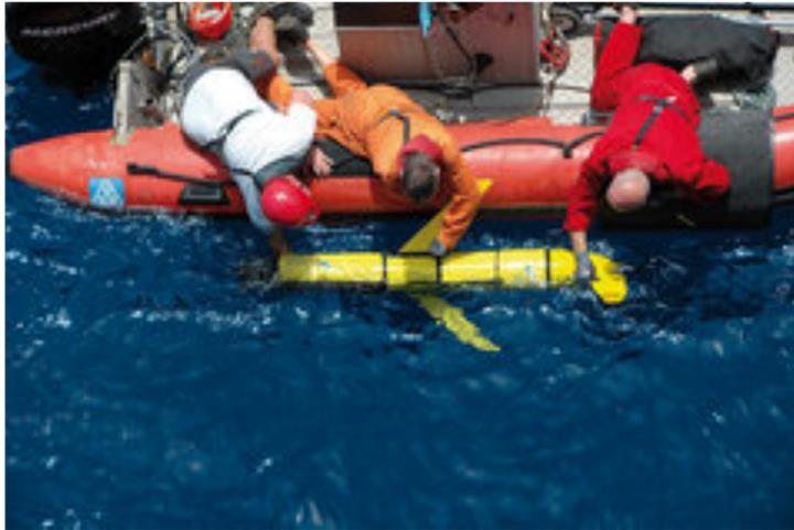
*Glider deployment with Rubber Boat – the usual procedure*
